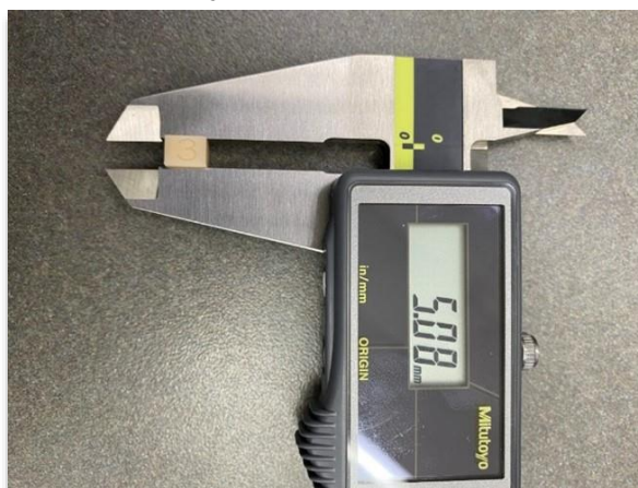
Figure 11. Calipers measuring calibration Cube 3.
